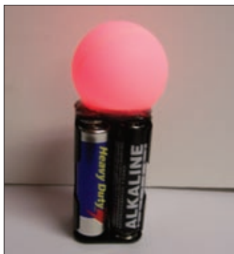
Fig. 1. The tri-color Ping-Pong ball color mixer.
